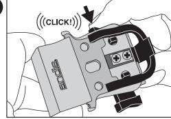
Push the button on the right of the locking arm to lock into place. The button should click into place.
