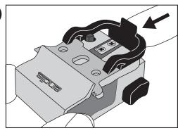
Push the upper blade adjustment bracket forward as far as it will go until the upper blade is firmly against the angled metal surface.
