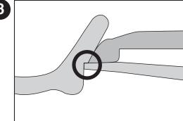
Make sure that the blade is properly seated against the lip of the blade gapper.
