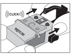
Place front end of blade under lip of blade gapper. Place holes on the blade assembly onto the pins of the blade gapper and pull back on the base of the blade. The front of the blade should lift up and click into place.
