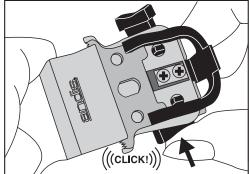
Release the blade lock by pressing the button on the left side of the locking arm. The button should click into place.
