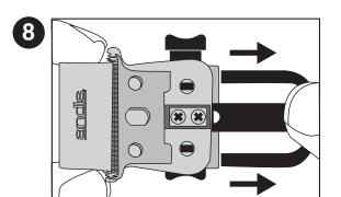
Pull the upper blade adjustment bracket back to release the blade set. Your blade set is now zero-gapped.
