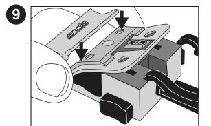
Remove blade assembly by pushing down on the front of the blade.
